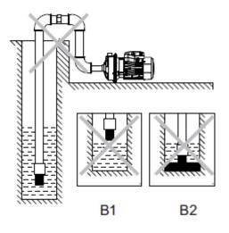
While installing the pump, use correctly rated suction tube for the inlet pipeline
