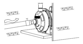
For pump installations, the inlet (or suction) pipe should be as short as possible with the least number or bends. The pump should be installed in a ventilated environment. It could be installed outside, provided the pump is adequately covered from the elements.
